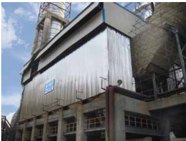
Figure 1. Double row filter type IFJCN 80/48-8000 D ECO at the Rauri cement plant, Himachal Pradesh, India.
