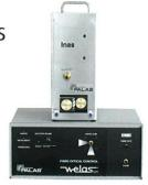
Palas's welas digital 2000/3000 light-scattering spectrometer system, which determines particle concentration and size precisely and reliably. Hall 6, Booth 109
