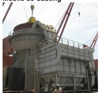
Intensiv-Filter has commissioned three further mobile dedusting devices for the ship unloading and truck loading in the harbour of Tema, Ghana. The bag filters complement an already existing mobile dust removal device. With it the capacity can be raised by a further volume flow of 44,000 m<sup>3</sup>/h. The filter surface amounts to additional 388 m<sup>2</sup>.
