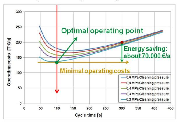
Prediction of the optimum cycle time as a function of the applied air tank pressure by the filter expert system ProExpertise, case study: high dust kiln / raw meal mill bag filter, ProJet mega<sup>®</sup>, 8 m bag length
