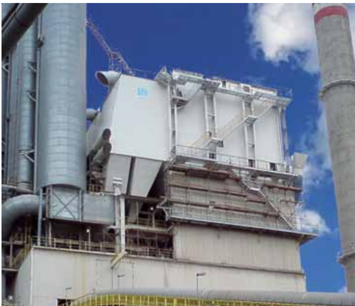
Nowiny, Poland (Dyckerhoff) Electrostatic filter conversion Two CombiJet double row filters with offline cleaning Dust removal in a rotary kiln
