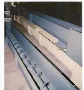
Dust discharge screw.
