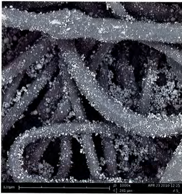
Figure 5. REM images (x1000) of filter media surfaces after testing in accordance with VDI 3926: ProTex PMIA (l.), ePTFE membrane (r).
