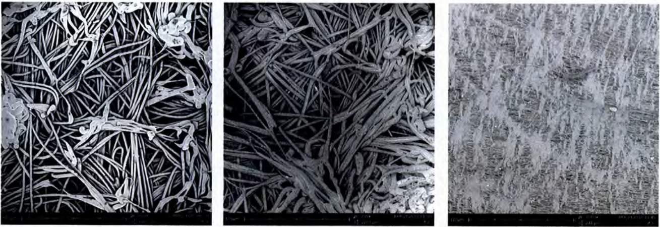
Figure 1. REM images of filter media surfaces: ProTex PES x200 (l.); ProTex PMIA x200 (m.); ePTFE/membrane x1000 (r).
