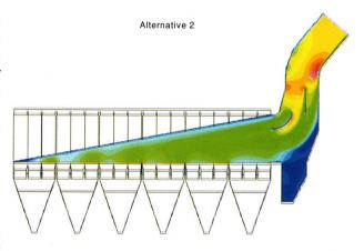
Using CFD, the second alternative shows clearly which optimisations are achieved with constructive changes. After evaluating and analyzing the CFD data, buffle plates are placed at the most optimal positions. The construction of the raw gas inlet is enhanced due to the CFD-simulations.
