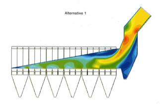
Using the example of the inlet stream, alternative one shows the initial situation of the dust removal installation.
